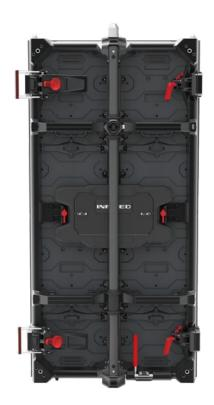
The separate power and data units can be easily exchanged with no tools required.
